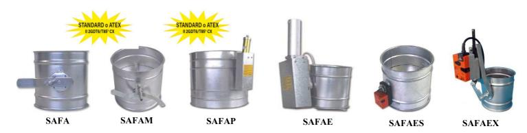
The butterfly shutters until  $\emptyset$  480 are galvanized or stainless steel made with a modular system that allows to change the way to open them just changing the outside mechanism without taking off the shutters from the aspiration system (manual, equalizer, pneumatic or electric).
